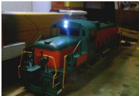
There are a number of applications for LEDs in our hobby. You can make your own flashing FRED unit, illuminate interiors, ditch lights for diesels, the list is endless. Go out and give it a try!
